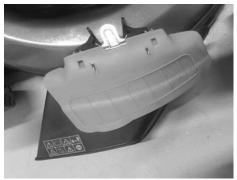
NOTE: Before installing the side discharge, remove the grass catcher. Both functions cannot be used together in the same time.
