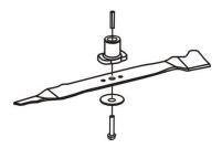
To remove the blade, loosen the screw, check the blade bracket, and replace all parts if they are worn or damaged.
