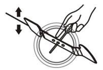
The blade is made of hardened steel. To get a clean job, sharpen the blade frequently, about every 25 hours of use. Make sure the blade is always well balanced. Insert a small iron pin (2 or 3 mm in diameter) into the hole in the middle of the blade: it must remain horizontal. If the blade does not stay horizontal, balance it by sharpening it further on the side where it is leaning.
