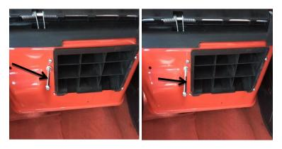
To use the back discharge function you must open the ejector flap slightly. The mulching adapter is not allowed to be fitted when the rear ejector is used.
